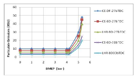
Figure 4: Variation of Particulate Emissions in Hartridge Smoke Unit (HSU) with Brake Mean Effective Pressure (BMEP) in Conventional Engine (CE) and Engine with LHR Combustion Chamber at Recommended Injection Timing and Optimum Injection Timing and at an Injector Opening Pressure of 190 Bar with Biodiesel (BD)
