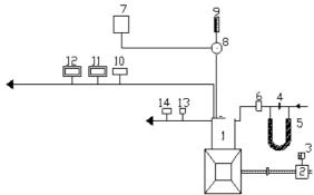
Engine, 2. Electical Dynamo Meter, 3. Load Box, 4. Orifice Meter, 5. U-Tube Water Manometer, 6. Air Box,
