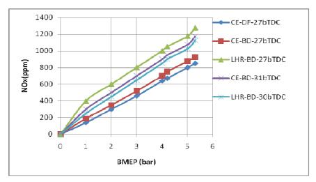
Figure 5: Variation of Nitrogen Oxide Levels with Brake Mean Effective Pressure (BMEP) in Conventional Engine (CE) and Engine with LHR Combustion Chamber at Recommended Injection Timing and Optimum Injection Timing and at an Injector Opening Pressure of 190 Bar With Biodiesel (BD)
