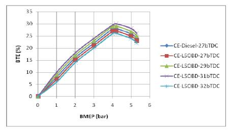
Figure 2: Variation of Brake Thermal Efficiency (BTE) with Brake Mean Effective Pressure (BMEP) in Conventional Engine (CE) and with Various Injection Timings at an Injector Opening Pressure of 190 Bar with Biodiesel
